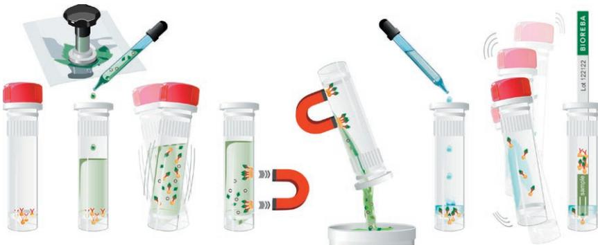
A plant extract is first incubated with magnetic beads coated with pathogen-specific antibodies. These beads are then separated from the extract with a magnet and resuspended in a small volume of running buffer. Finally, a strip is inserted and the concentrated beads migrate upwards through the strip and brown colored lines will become visible.
